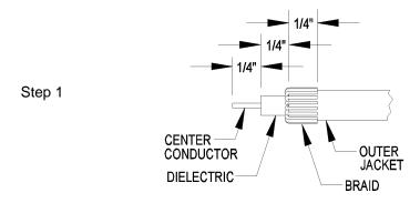
Prepare the cable according to step 1 to achieve the proper braid exposure and center conductor length. Fold the braid against the outer jacket as shown. Twist the foil tightly against the dielectric and verify there are no loose braids or foil touching the center conductor.
